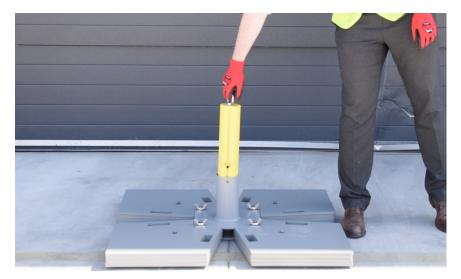
Ensuring that the pin hole of the abseil post and abseil base are aligned, insert an Mx12 quick release pin through the base and abseil post. **THIS IS A SAFETY CRITICAL OPERATION. PLEASE CHECK THE PIN HAS DEPLOYED.**
