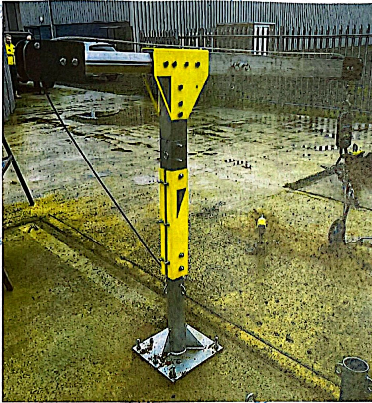
Figure 1 – Anchor described as "1500 x 1500 davit arm"
